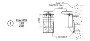
CHAMBER TOO LOW — CONNECT -EZ CAN PROVIDE A CUSTOM STUB COLUMN AND CONCRETE ANCHORS TO SUPPORT JOIST AT DESIGN ELEVATION.
