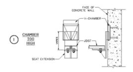
CHAMBER TOO HIGH — CONNECT -EZ CAN PROVIDE A CUSTOM SEAT EXTENSION TO SUPPORT THE JOIST AT THE DESIGN BEARING ELEVATION
